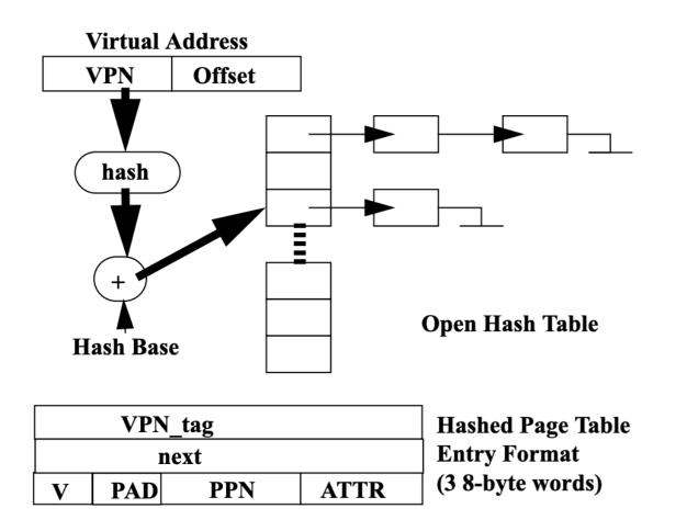
In HPT, the Virtual Page Number (VPN) is hashed into a key. The key can be used (together with the Base) to index the HPT to find the PPN (Physical Page Number).
