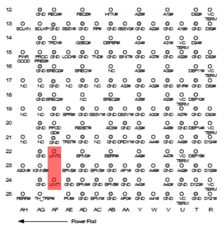
LINTx — lines/pins for hardware interrupts.
