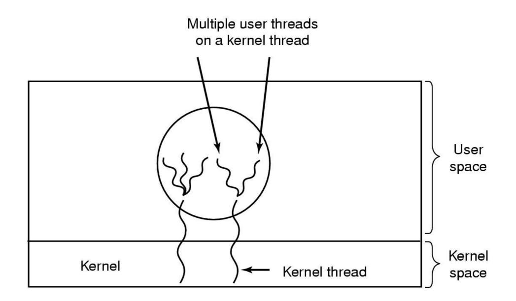
M:N model multiplexes N user-level threads onto M kernel-level threads Good idea? Bad Idea?
